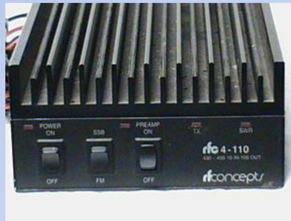
RF Concepts rfc4-110, 432 MHz 10 w in, 100 w out
