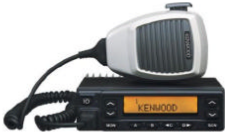
Kenwood TK-981 commercial radio easily programmed for 927.5 MHz FM, ~$130
