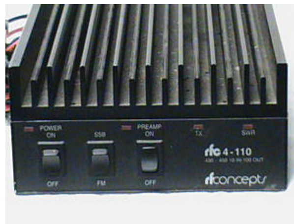
RF Concepts rfc4-110, 432 MHz 10 w in, 100 w out
